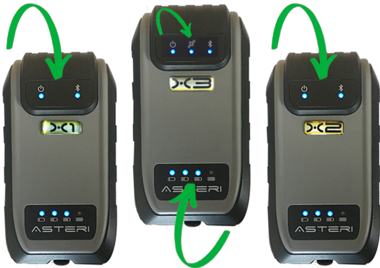
The different LED status indicators on the Asteri GNSS receiver
