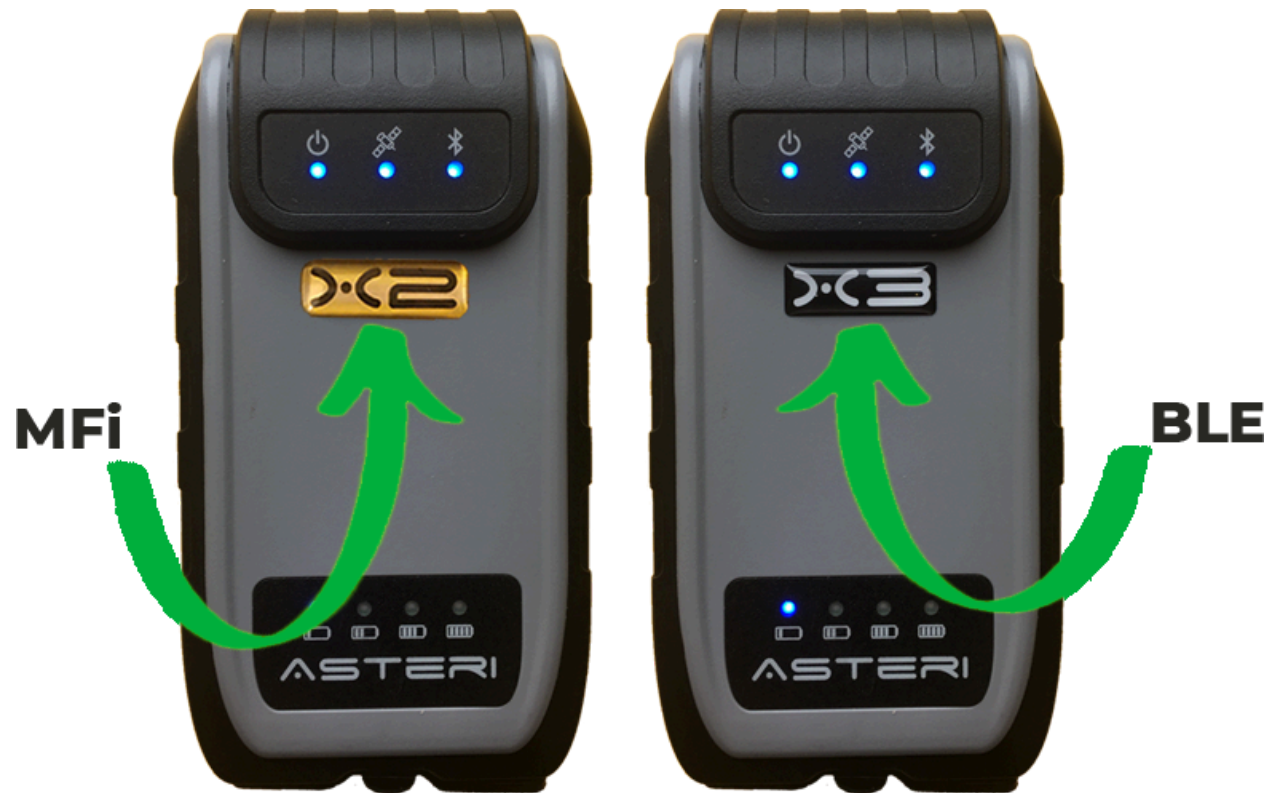
The Gold labeled MFi model compared to the Black labeled BLE model
